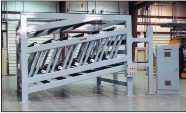
This example of a custom PDG is of a six web pedestal AccuGuide PDG-FS for a sheeter application.
